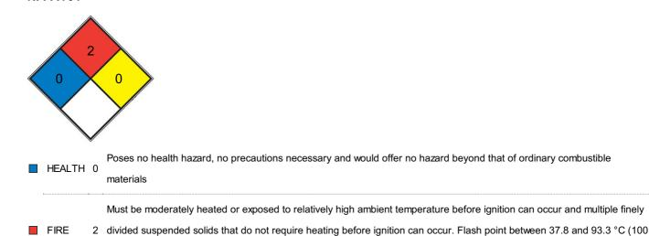
REACT 0 Normally stable, even under fire exposure conditions, and is not reactive with water (e.g. helium, N2)
