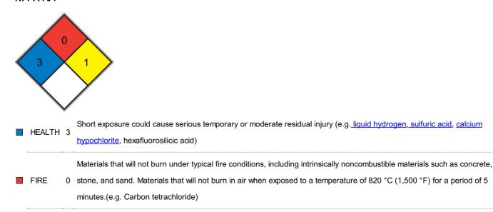
1 Normally stable, but can become unstable at elevated temperatures and pressures (e.g. propene)
