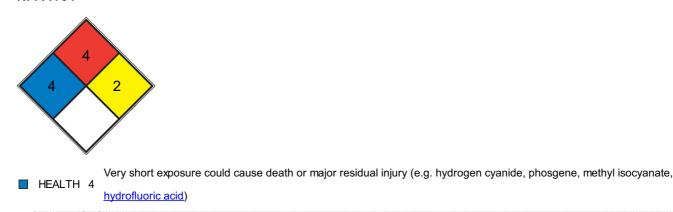
Will rapidly or completely vaporize at normal atmospheric pressure and temperature, or is readily dispersed in air and will FIRE 4 burn readily. Includes pyrophoric substances. Flash point below room temperature at 22.8 °C (73 °F). (e.g. acetylene,
