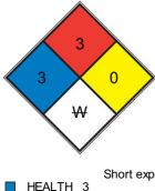
Short exposure could cause serious temporary or moderate residual injury (e.g. <u>liquid hydrogen, sulfuric acid</u>, <u>calcium</u> <u>hypochlorite</u>, hexafluorosilicic acid)
