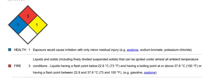
REACT 1 Normally stable, but can become unstable at elevated temperatures and pressures (e.g. <u>propene</u>)
