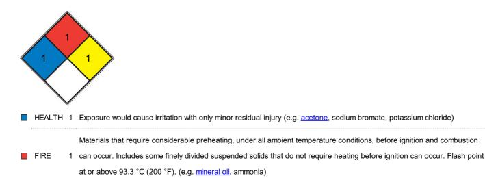
REACT 1 Normally stable, but can become unstable at elevated temperatures and pressures (e.g. propene)
