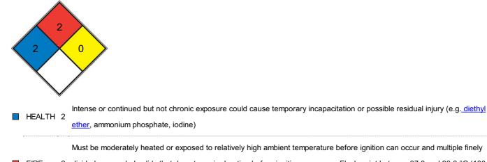
FIRE 2 divided suspended solids that do not require heating before ignition can occur. Flash point between 37.8 and 93.3 °C (100 and 200 °F). (e.g. diesel fuel, sulfur)
