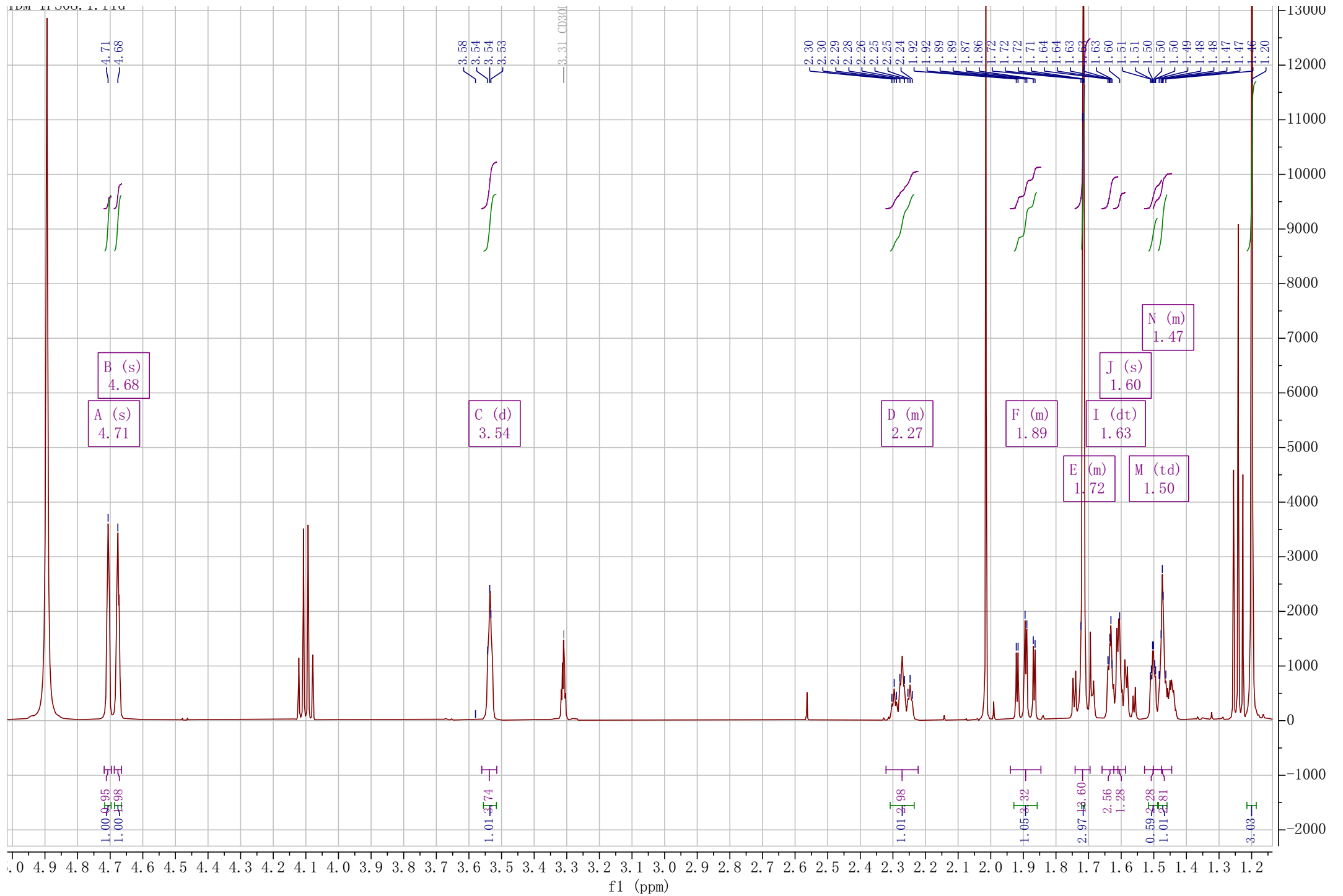
1 H NMR (500 MHz, Methanol- d 4 ) δ 4.71 (s, 1H), 4.68 (s, 2H), 3.54 (d, J = 3.2 Hz, 4H), 2.32 – 2.22 (m, 3H), 1.94 – 1.85 (m, 3H), 1.73 – 1.70 (m, 14H), 1.63 (dt, J = 3.4, 1.7 Hz, 3H), 1.60 (s, 1H), 1.50 (td, J = 3.2, 1.4 Hz, 2H), 1.49 – 1.46 (m, 3H)
